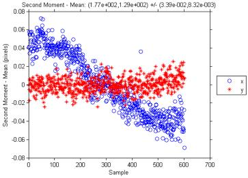
Finally, we measured the overall beam tilt at each of these measurements. The variation in the tilt again showed a slight pattern to the data, which was reflected more clearly in the x-axis data than the y-axis. The measured tilt standard deviation was 5.6 and 0.77 µrads in the x and y axes respectively.
