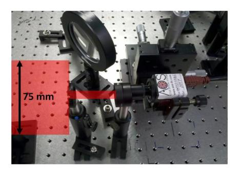
Each wavefront sensor was setup such that the intensity was >90% of the total intensity dynamic range by keeping the black level at 16 and the gain at its lowest setting and adjusting the exposure length. We consistently used a 10% threshold on centroiding for spot location determination. We also always acquired a full frame (typically  $640 \times 480$  pixels) at the highest frame rate (typically 60Hz).
