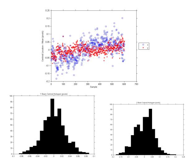
The second moment of the overall beam was calculated for each of the frames as well. There appeared to be an overall trend to the x second moment data despite our attempt to minimize any change in the experimental setup during these runs. The standard deviation of the second moment measurements was 0.034 and 0.0083 in the x and y axes respectively. The y-axis second moment variation was fairly Gaussian, but the x-axis data was affected by the trend.
