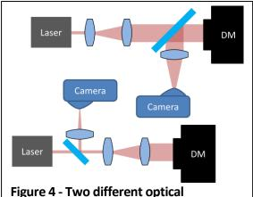
Figure 4 - Two different optical configurations that are commonly used for beam shaping experiments
