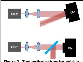
Figure 2 - Two optical setups for quickly determining deformable mirror functionality
