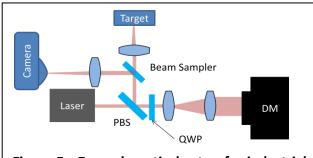
Figure 5 - Example optical setup for industrial beam shaping applications
