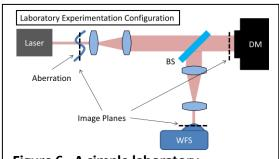
Figure 6 - A simple laboratory configuration for doing basic AO testing
